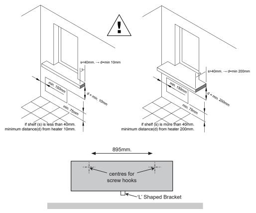
Locate the appliance over the top of the screw hooks and allow it to hang in place.
